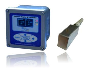
The Alpha2000 is an Ultrasonic Doppler Flowmeter consisting of a transmitter, a clamp-on transmit/receive sensor, The transmitter's electronics is specifically designed to analyze, separate and reject noise frequencies. The ultrasonic sound waves are coupled from the sensor, through the pipe walls and are reflected off the particles in the fluid and back through the pipe walls to the sensor.
